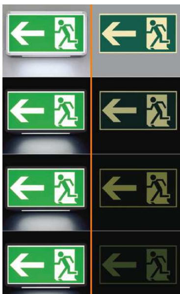
Below: Comparison between internally illuminated exit signs and PL exit signs shown before Power failure and then at 10minutes, 30 minutes and 60 minutes after power failure
